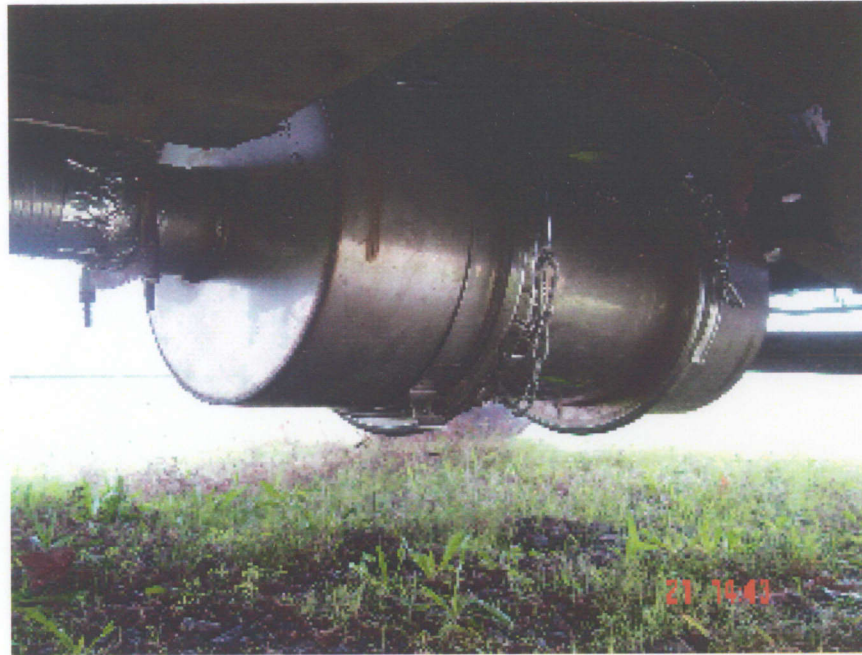
Figure 10: Lubrizol Purifilter installed into the exhaust system of a T444E engine prior to mobile emissions testing.
